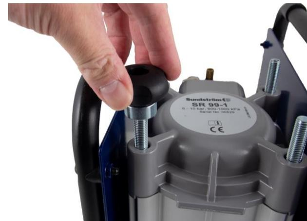
2.10 Tighten the knobs alternately by hand until the lid meets the filter housing.
