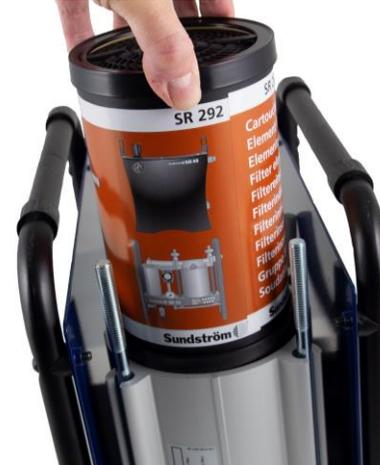
**2.6** Mount the new filter element. This has identical ends and can be fitted either way round.
