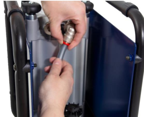
**2.2** Loosen the hose between the regulator and filter lid by pushing the red sleeve on the coupling and disconnect the hose from the lid.
