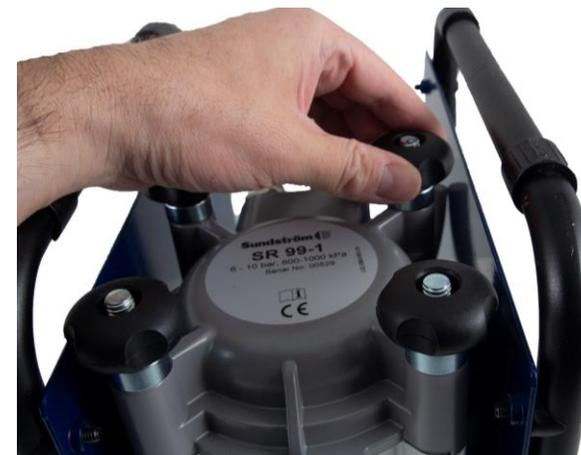
**2.3** Unscrew the knobs of the filter housing and remove the lid.
