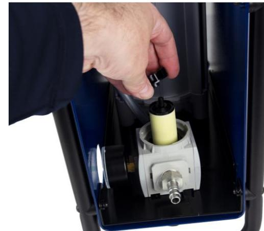
**4.3** Blow the parts clean with compressed air. Check that the drain outlet is not obstructed.
