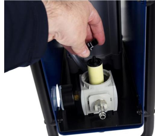
**3.3** Remove the pre-collector element by turning it anti-clockwise.
