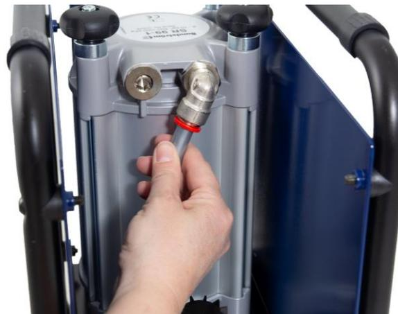
2.8 Connect the hose between the control valve and filter lid by pushing the hose into the connector.
