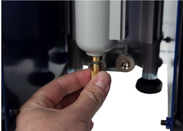
**1.3** The filter is automatically drained to the given level. The drain can also be opened manually by turning the pre-collector at the bottom of the drain bowl.
