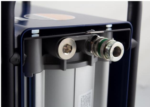
**1.1** The filter has two outlets one of which is plugged prior to delivery.
