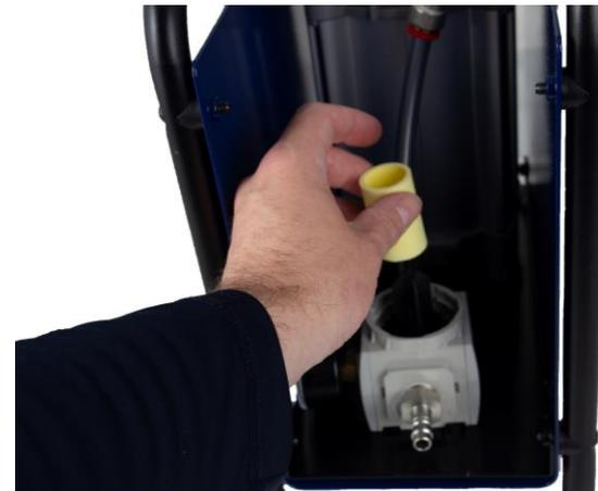
**3.4** Blow the parts clean with compressed air. Check that the drain outlet is not obstructed.
