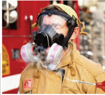
**Irritant smoke is the only OSHA-accepted qualitative fit testing method that does not rely on the test subject's subjective response.**
