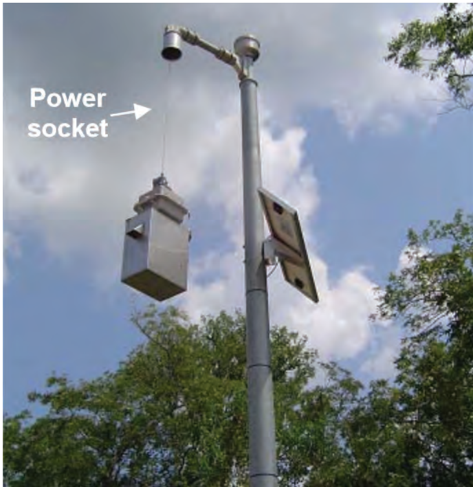
Figure 3. Lowering the AreaRAE for service using the flagpole-type cable.
