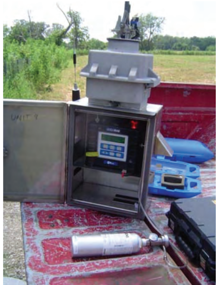
Figure 5. AreaRAE lowered for calibration.
