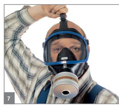
... tighten front strap if necessary.
