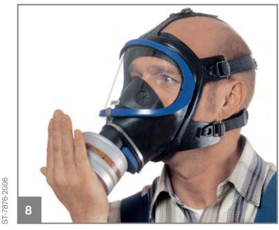
Negative pressure test: Seal respiratory filters with your palm and breathe in until a negative pressure (suction) is generated. Hold your breath for a mo-ment. The negative pressure should be maintained. If not, readjust the face piece and adjust the straps. Repeat test until a successful for check is met. Warning: Beards in the sealing area of the mask can cause leaks. Always make sure the mask forms a tight seal and the filter is attached prior to entering a hazardous atmosphere.
