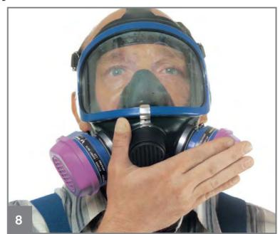
Positve pressure test: Seal off the protective cap of the exhalation valve with your palm and exhale. The mask will inflate slightly. If the mask does not inflate slightly, readjust the face piece and adjust headstraps or use a different mask size. Repeat the test until a successful fit check is met.
