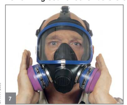
Negative pressure test: Seal both respiratory filters with your hands and breathe in until a negative pressure (suction) is generated. Hold your breath for a moment. The negative pressure should be maintained. If not, readjust the face piece and adjust the straps. Repeat test until a successful fit check is met.
