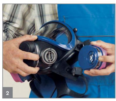
Use markings on the mask body and filter to help align the filter.
