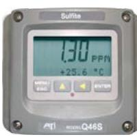
ATI's Model Q46S/66 Residual Sulfite Monitor provides the solution to dechlorination control in wastewater effluent. The sample stream is acidified which converts the sulfite ion into sulfur dioxide. The air-stripping system removes the sulfur dioxide from the solution and is measured with a gas-phase SO<sub>2</sub> sensor.
