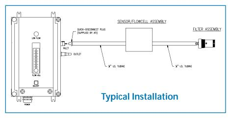
The type of tubing used on the portion of the sampling system between the sample point and the inlet port of the gas sensor is another important consideration. Reactive gases require the use of Teflon or other fluorocarbon tubing, while non-reactive gases can be sampled using flexible PVC tubing. Sampling from gas streams saturated with moisture may require heated sample tubing, and the effect of condensation on the gas sensor must be carefully evaluated.
