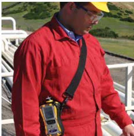
MultiRAE used for worker exposure monitoring at an oil refinery
