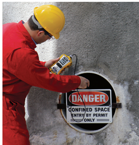
Confined space testing with the MultiRAE Lite
