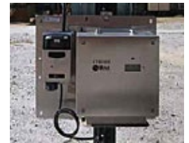
PowerPak connected to MeshGuard monitor. Monitor is shown in protective stainless-steel housing, secured with included hardware.
