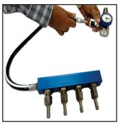
Fig. 2: Inserting manifold nozzle to Pressure reducer coupling
