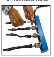
Fig. 4: Inserting detector tube holder in manifold port
