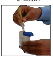
Fig. 5: Breaking off detector tube tips
