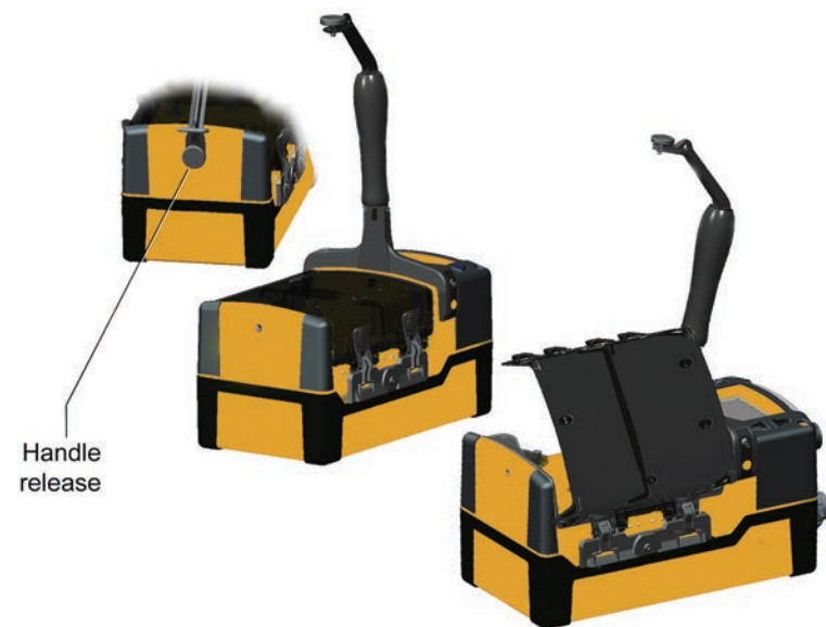
Figure 8: Opening the Chemcassette cartridge door
