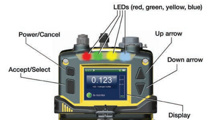
Figure 2: SPM Flex buttons and color LCD display
